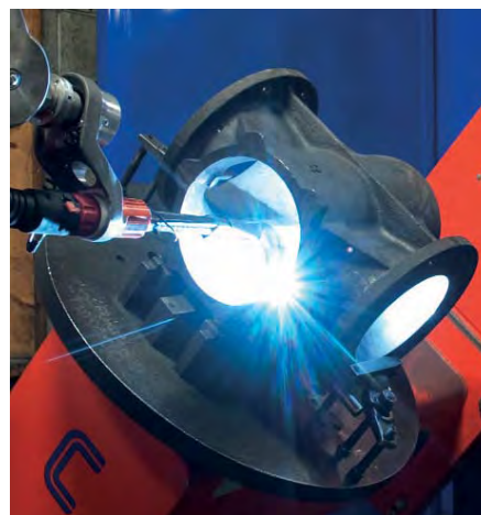
Figure 3. Robotic welding of nickel seat
